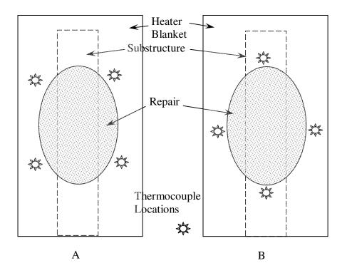
Figure 1. A schematic representation of the influence of alternative thermocouple placements on repair outcomes.
