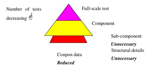
Figure 3. A reduced certification test program where the adhesive bond load capacity is designed to always exceed the structural loads.
