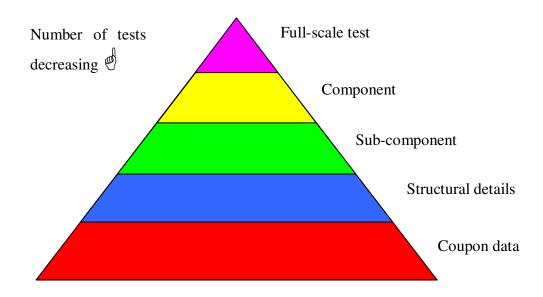
Figure 2. A schematic representation of the building block approach to certification of adhesive bonded structures.
